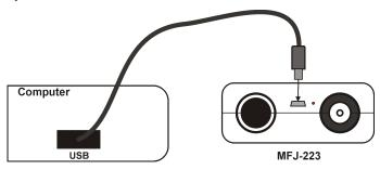
To monitor the charge cycle, check the status LED located to the left of the charging jack (LED not visible unless charging is in progress). <u>Red LED</u> signals normal charging, <u>Green LED</u> indicates when charging is complete, and <u>Flashing LED</u> warns of a charging fault (battery or power-source problem).
