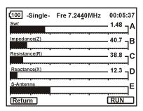
With the generator running, you may change frequency on the fly using the Encoder while watching the display for key points of interest such as resonance (X = 0), minimum SWR, and the antenna's 2:1 bandwidth limits. You may also use the analog bars to provide continuous feedback when adjusting tunable circuits or matching networks. Pressing  $\underline{Run/Stop}$  again toggles the generator off.
